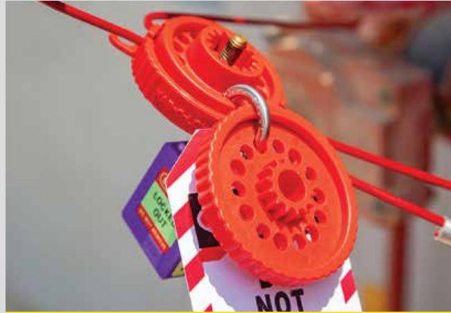
KAB-O-LOK's Operating Tool has been designed to lock into the device. The USP and salient feature of the Operating Tool allows the tool to be locked into the base unit. Locking the tool into the last base unit ensures tool can never be misplaced or lost and remains on site for the re-energization process.
