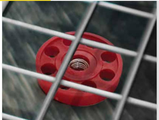
The PRO-LOCK® device does not include this feature. The tightening wheel comes off and falls into crevices on rigs & offshore platforms, making it unretrievable. This renders the device inoperable, increasing downtime during shutdowns.
