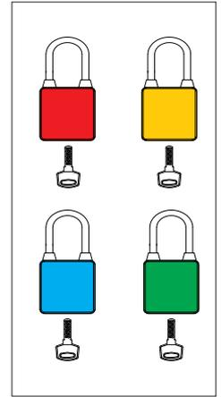
**KEYED DIFFERENT (KD)** padlocks cannot be master keyed. If key is lost or misplaced, the padlock has to cut/destroyed.
